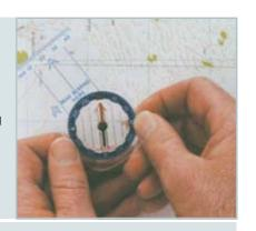
Put the map aside. Hold the compass steady and level in front of you with the Direction of Travel Arrow pointing straight ahead. Turn your body until the red end of the Needle is directly over the Orienting Arrow, pointing to the "N" on the dial. The Direction of Travel Arrow now points to your destination. Look up, align the Direction of Travel Arrow with a feature and walk to it. Repeat this procedure until you reach your destination.
